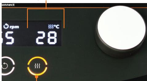
Heating button: Heating on
